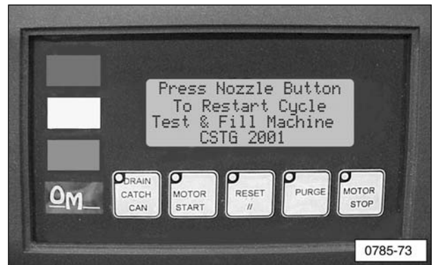
Illustration 12. Alternate Display After Test Tube Or Undercarriage Component Is Successfully Filled With Oil.
