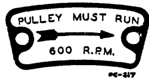
Figure 5 Main Drive Pulley Must Rotate in This Direction Viewed From Rear of Machine
