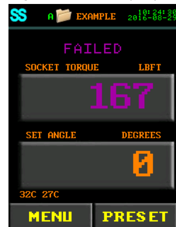
Figure 7.2-4: Failed Torque Cycle with Smart Socket Result
