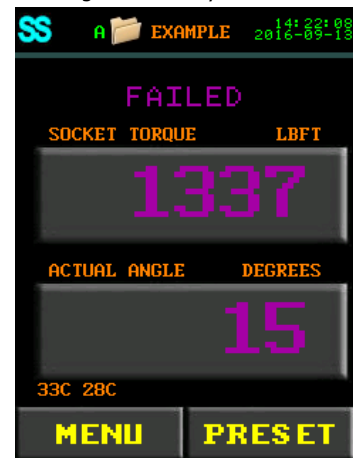
Figure 7.4-5: Failed Torque and Angle with Smart Socket
