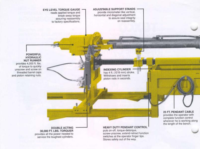
When your business is repairing hydraulic cylinders, versatile, easy to use, powerful and well designed equipment is the key to getting the job done fast and profitably. And that's what TUXCO's new HCS-30 Hydraulic Cylinder Servicer is all about – one man operation and greater efficiency and more profit.
