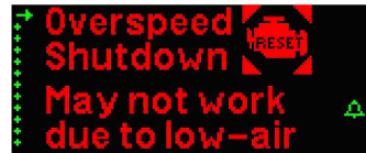
Engine Over-Speed Shutdown Low Air Warning
