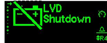
Low Voltage Disconnect
