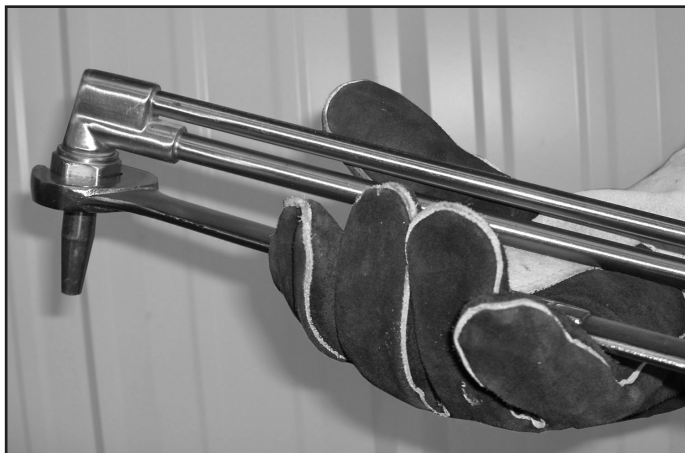
Figure 17: Tightening the Tip Nut
