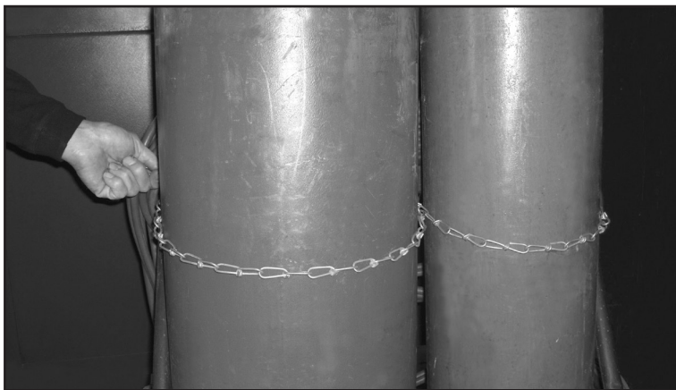
Figure 8: Securing the Cylinders in the Cart
