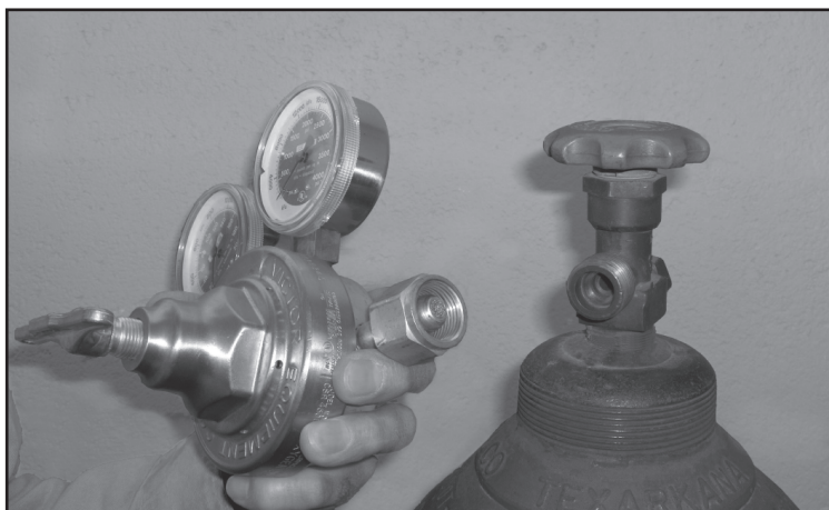
Figure 9: Inspecting the Cylinder and Cylinder Valve
