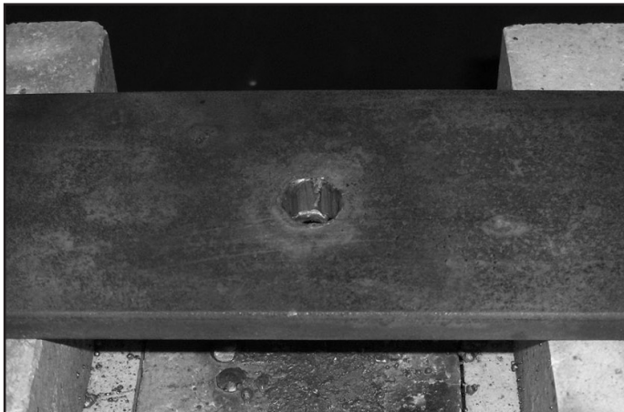
Figure 22: Cutting by Piercing
